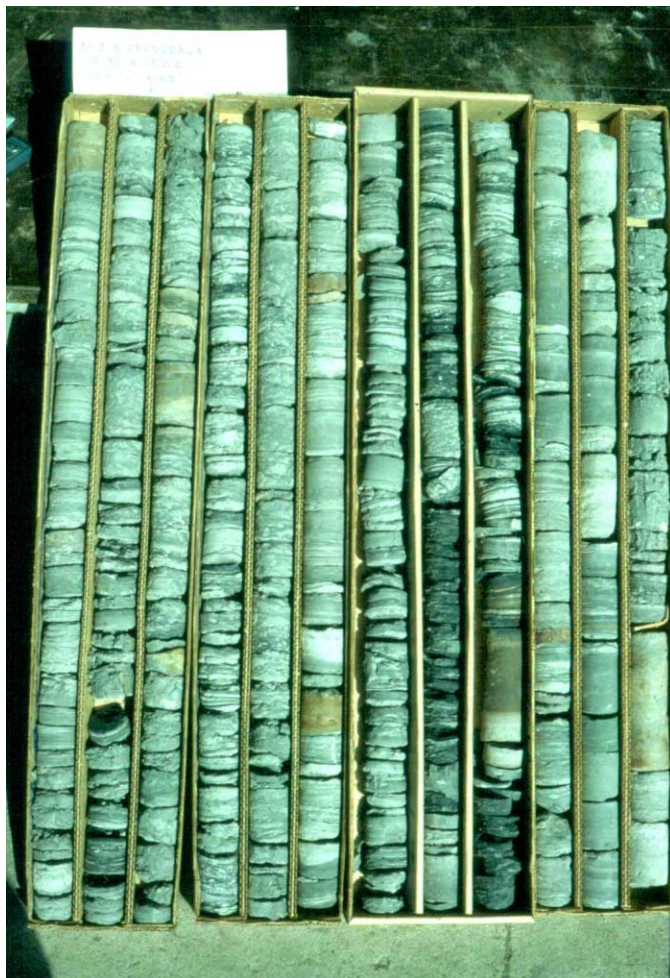
Figure 44 – Bioturbated sandstone in Unit 1 of the Pense Formation at Mobil South Grassdale 32-10 (10-32-6-15W2), southeastern Saskatchewan.
