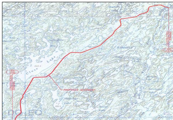
The proposed roadway is 51.71 km in length. The proposed location was established while considering existing terrain, Ministry of Highways and Infrastructure (MHI) geometric standards, and Ministry of Environment (MOE) setbacks from water bodies.
