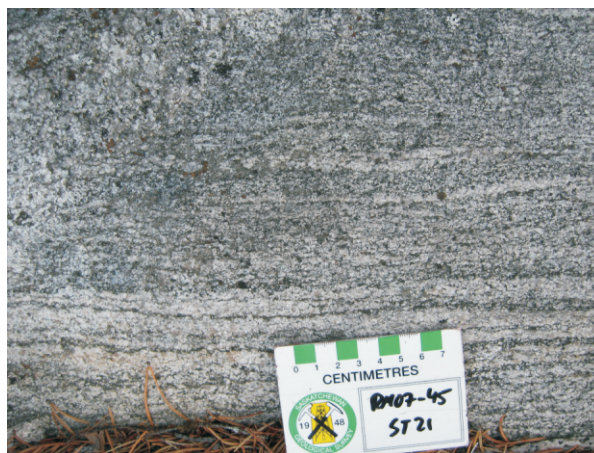
Figure 17 - Granodiorite-tonalite with well-developed gneissic layering; west shore of Kakinagimak Lake just south of Cornell Bay. Station RM07-45-ST21 at UTM 672077 m E, 6120368 m N.
