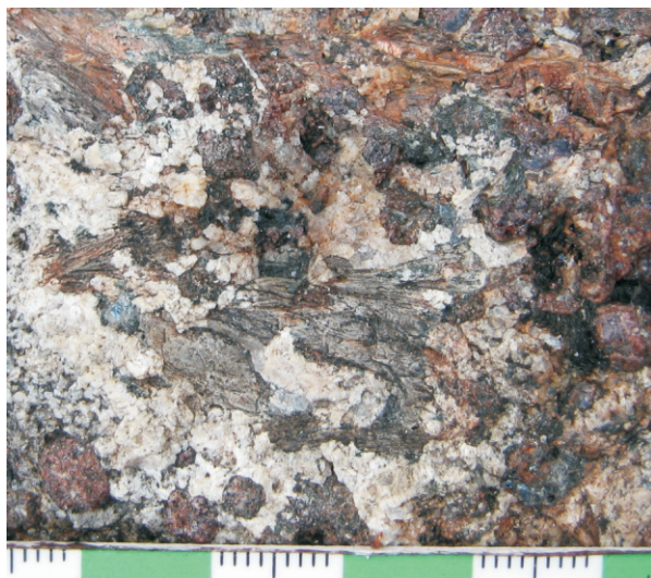
Figure 22 - Garnet-anthophyllite alteration in felsic volcanic rocks; east central Keep Lake. Station RM07-48-ST19 at UTM 676265 m E, 6111989 m N.
