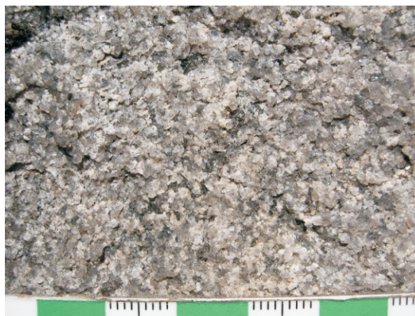
Figure 19 - Magnetite-garnet-quartz-rich diatexite, possibly derived from Missi Group feldspathic psammite; northwest of McWilliams Lake. Station RM07-12-ST02 at UTM 668161 m E, 6112337 m N.
