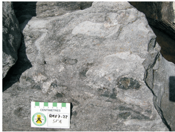
Figure 6 - Heterogeneous felsic volcanic rock; possibly a rhyolitic tuff breccia; rock has also been affected by silicification and calc-silicate alteration (note dark-coloured calc-silicate lenses); north Gifford Bay. Station RM07-22-ST08 at UTM 671954 m E, 6110192 m N.
