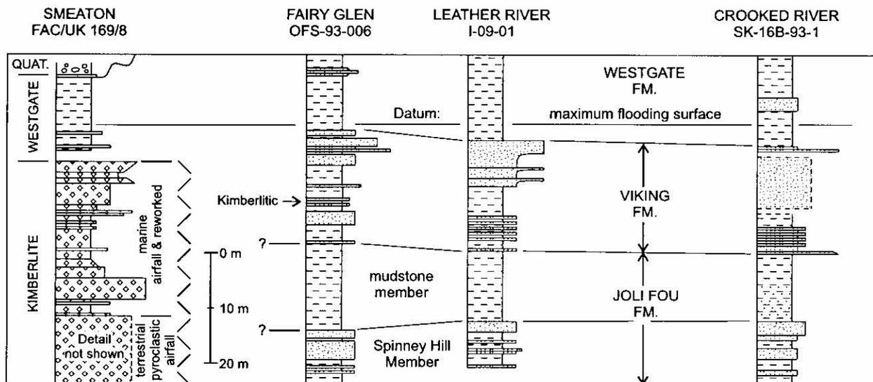
**Figure 3 - Stratigraphic position of kimberlite rocks in the Smeaton FAC/UK 169/8 core relative to Cretaceous stratigraphic units in the Fairy Glen, Leather River, and Crooked River cores. The maximum flooding surface within the lower Westgate Formation is drawn on the basis of microfossil data. A radiometric age of  $101.1 \pm 2.2$  Ma in the lower part of the kimberlite succession suggests that the kimberlites are of Viking age.**
