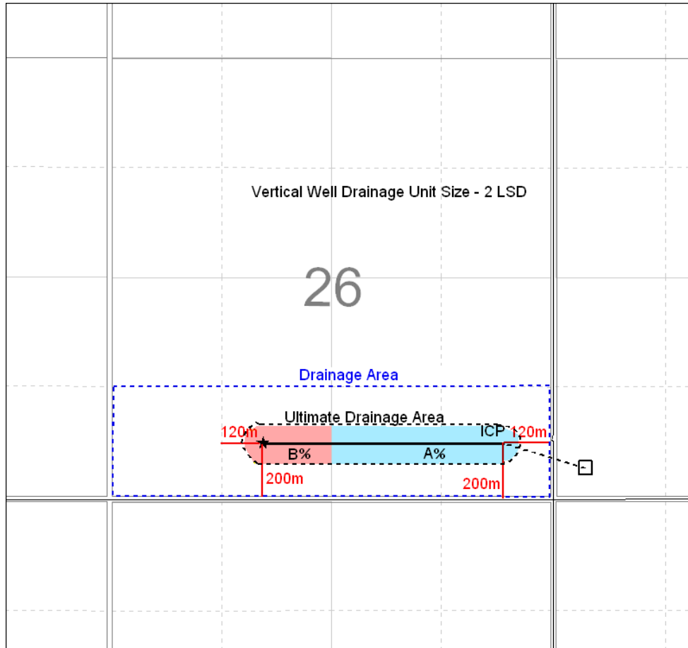
Figure 4. Determining the drainage area for a horizontal well with a Crown/freehold pooling agreement in place, where the vertical drainage unit area covers 2 legal subdivisions (LSDs).
