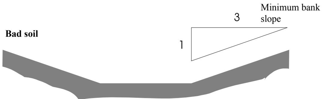
Type 4 soil must be sloped from the bottom of the excavation or trench, with a slope at an angle not steeper than three horizontal to one vertical, or  $19^{\circ}$  measured from the horizontal.
