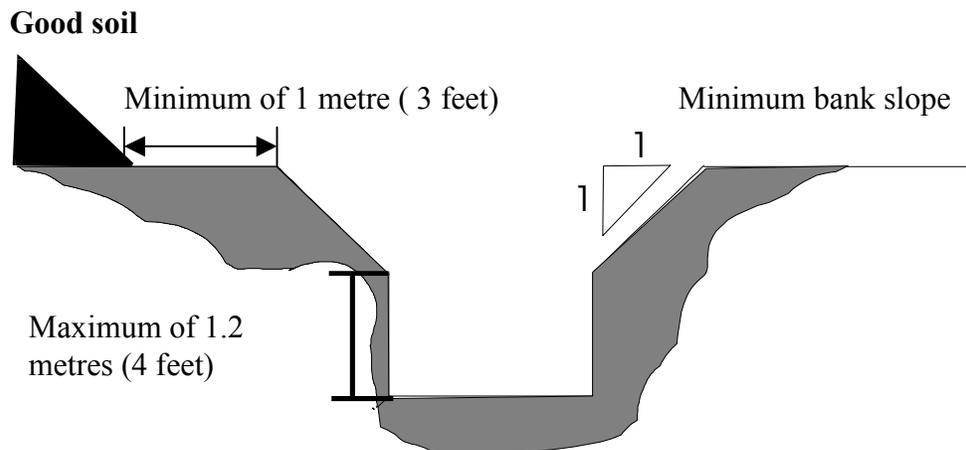
Type 1 and 2 soil must be sloped to within 1.2 metres (4 ft.) of the bottom of the excavation or trench, with a slope at an angle not steeper than one horizontal to one vertical, or  $45^{\circ}$  measured from the horizontal.
