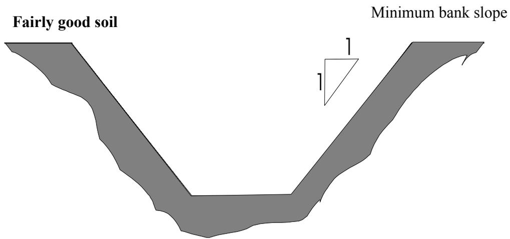
Type 3 soil must be sloped from the bottom of the excavation or trench, with a slope at an angle not steeper than one horizontal to one vertical, or  $45^{\circ}$  measured from the horizontal.
