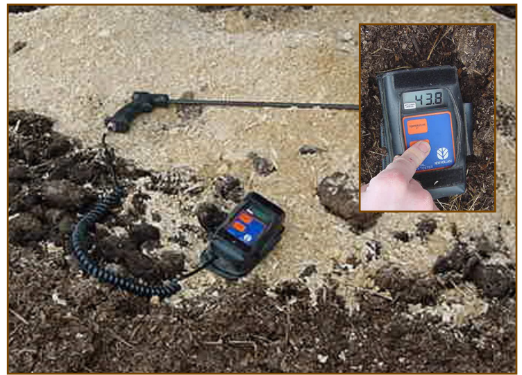
Figure 5: A hay moisture probe with a long stem works well to measure the moisture content of a compost pile. This pile is at the correct moisture level of about 45 per cent.
