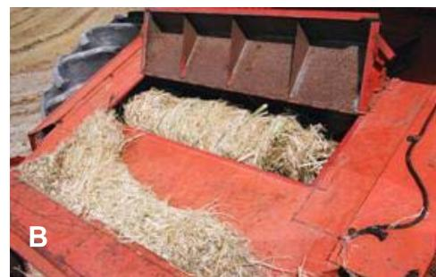
**Hemp fibre clogging the cutting bar (A) and combine paddles (B, swathed)** Courtesy of Hemp Oil Canada Inc.
